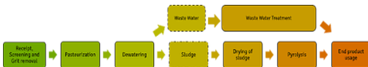
Community Scale Fecal Sludge and Septage Processor – Stages
